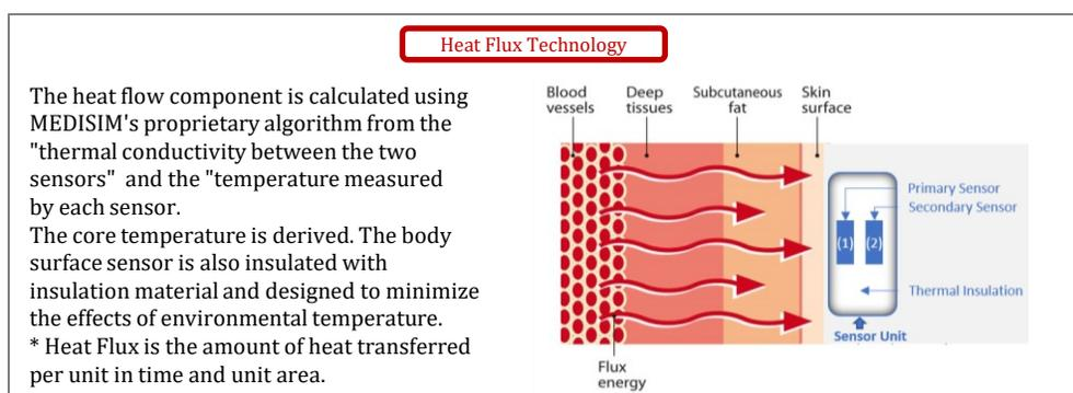
Figure 1: Measurement Method
