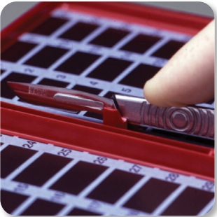
Step 2: Slide forward until blade “catches.”
