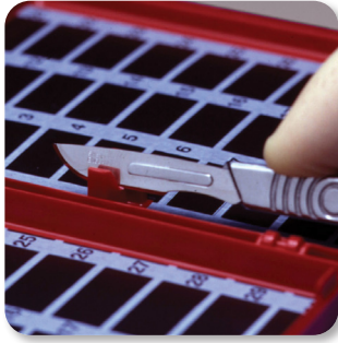
Step 1: Insert blade into DeBlade™ mechanism.
